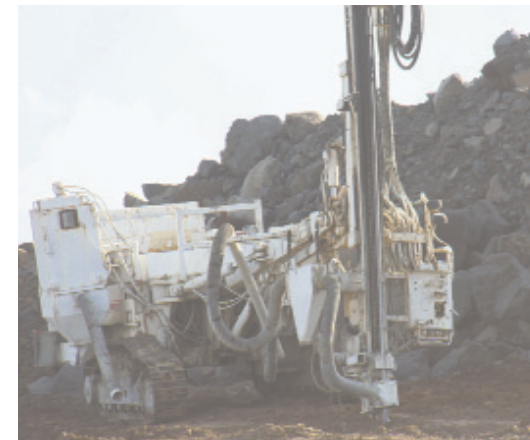
DRILL MACHINE used to drill holes in preparation for blasting.
